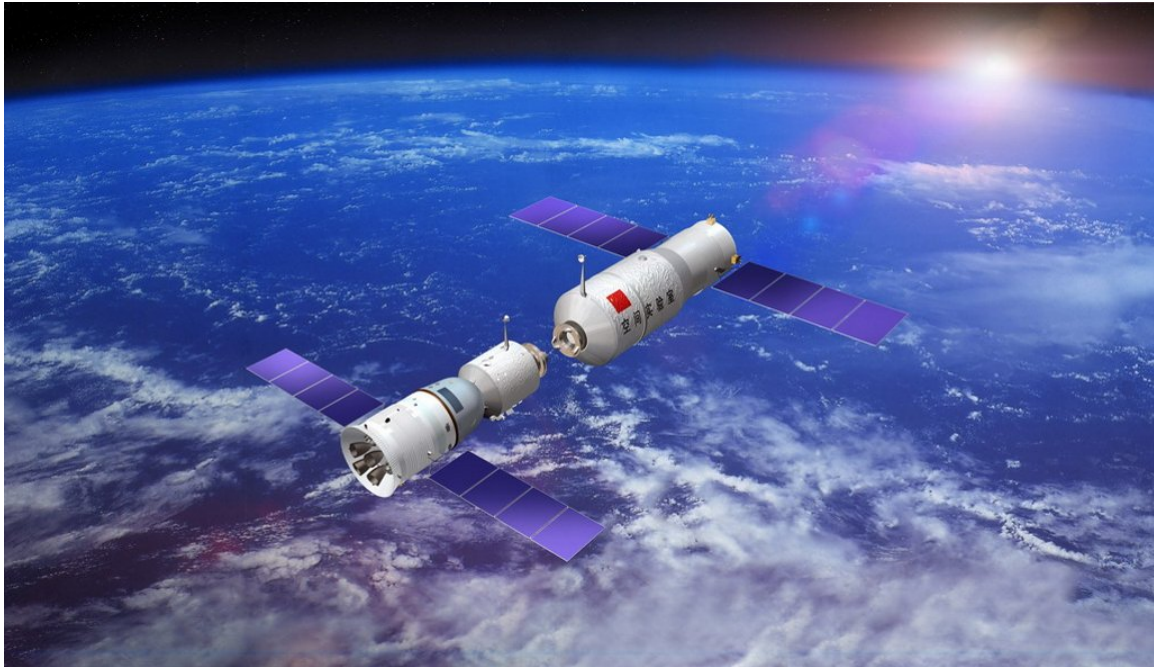
Fig. 2.2 Illustration of the unmanned, automated rendezvous and docking of the Chinese Shenzhou-8 spacecraft ( left ) with the Tiangong-1 module ( right ) which occurred on November 2, 2011. (China Manned Space Engineering Office photo).
