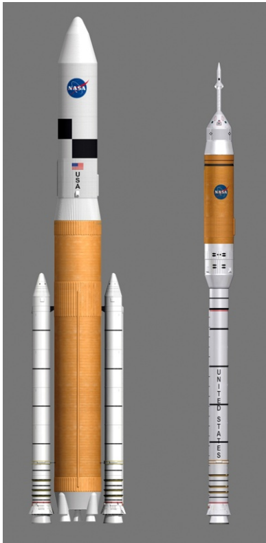
Fig. 5.6. A comparison of the Ares I (right) with the heavy-lift Ares V launch vehicles (left). Both rockets have been canceled, although data from the launch of Ares I-X ( Fig. 5.5 ) may be used for developing alternative rockets. (NASA photo).
